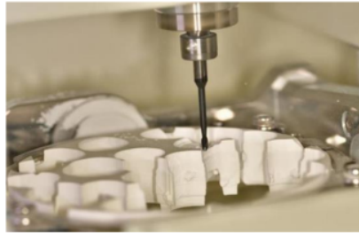
FIGURE 10. Computerized milling of the two prosthetic restorations in the zirconium dioxide disc.
