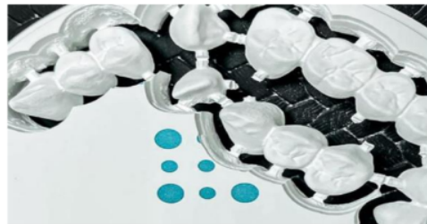
FIGURE 10. Computerized milling of the two prosthetic restorations in the zirconium dioxide disc.
