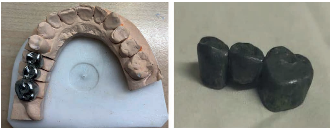
FIGURE 7. The metal framework processed and fitted on the functional model (a); the aspect of metal component at the end of the oxidation process (b)
