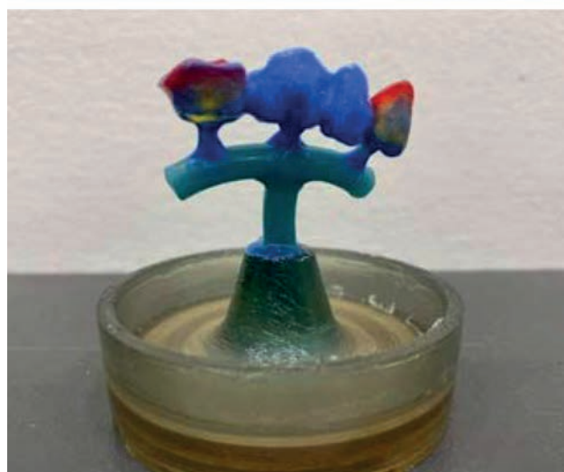
FIGURE 3. Preparing the wax-pattern for investing. Applying wax sprue rods (left), applying the wax pattern on the cone of the crucible former (right)
