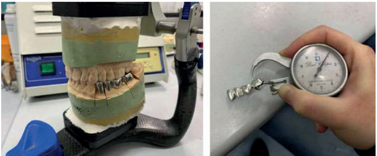
FIGURE 4. The final aspect of metallic framework on the working model (left). Checking the thickness of the dental alloy using a professional caliper
