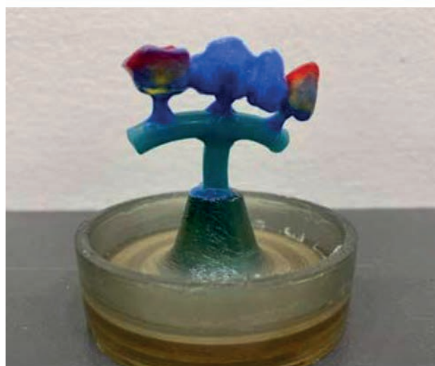
FIGURE 3. Preparing the wax-pattern for investing. Applying wax sprue rods (left), applying the wax pattern on the cone of the crucible former (right)
