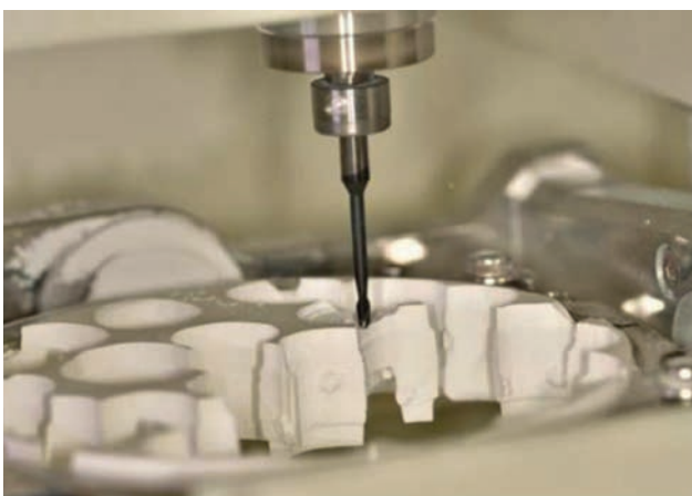
FIGURE 10. Computerized milling of the two prosthetic restorations in the zirconium dioxide disc
