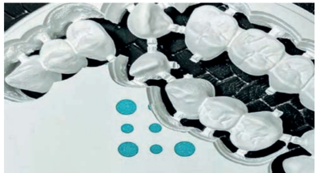
FIGURE 11. The appearance of the restorations at the end of the milling process
