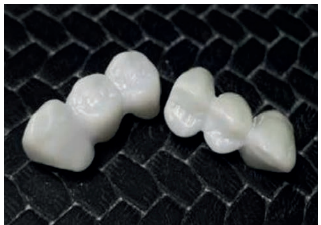
FIGURE 12. Prosthetic restorations at the end of the sintering program
