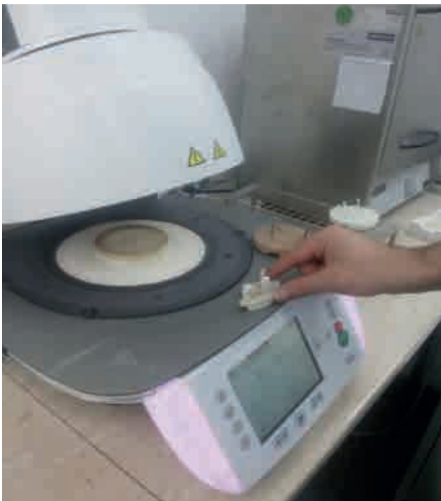
FIGURE 11. Ceramic veneer before firing in the ceramic furnace
