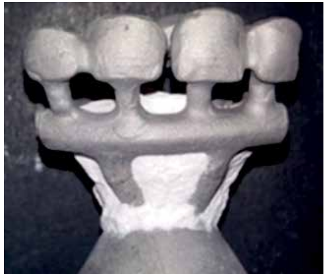
FIGURE 4. Metal framework after de-vesting
