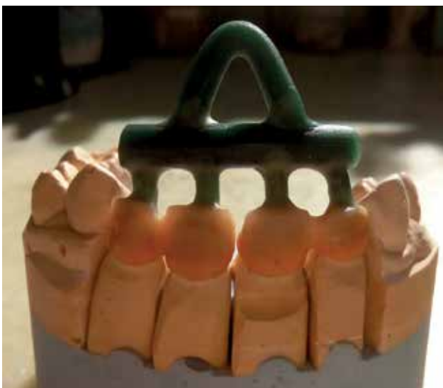
FIGURE 3. Rapid Wax system (Bego) attached to wax patterns prepared for investment [8]
