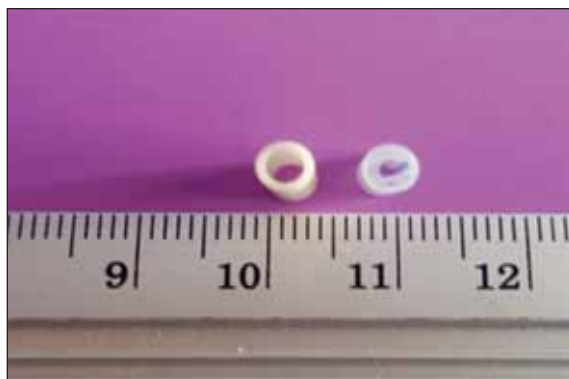
FIGURE 1. Polyurethane catheter (left) and silicone catheter (right) crossing section
